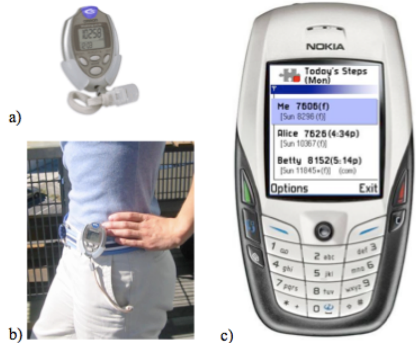
Figure 1. a) The Omron HJ-112 pedometer, b) the pedometer in use, and c) the Nokia 6600 mobile phone running Houston.
