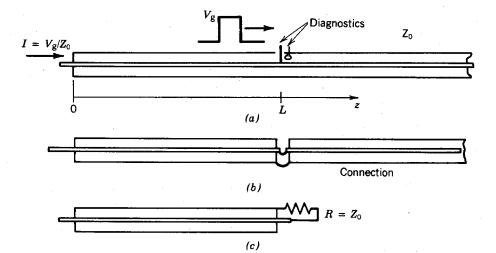
**Figure 9.31** Matched terminations of a transmission line. (a) Infinite length line with characteristic impedance  $Z_0$ . (b) Finite length line connected to a semiinfinite length line with the same characteristic impedance. (c) Transmission line terminated by a matched resistor ( $R = Z_0$ ).
