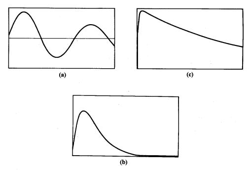
Figure 9.24 Voltage on a load driven by a switched capacitor with series inductance as a function of  $\beta/\omega_0$ : L and C constant, load resistance (R) varied;  $0 \le \omega_0 t \le 10$ . (a) Underdamped circuit  $(\beta/\omega_0 = 0.1)$ . (b) Critically damped circuit  $(\beta/\omega_0 = 1)$ . (c) Overdamped circuit  $(\beta/\omega_0 = 5)$ .
