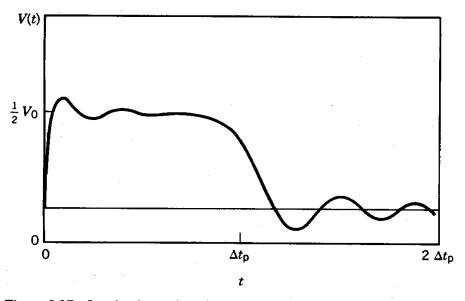
Figure 9.37 Load voltage, five-element PFN discharged into a matched load.
