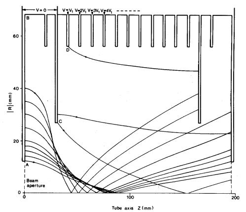
**Figure 9.22** Insulator column for a Van de Graaff accelerator showing orbits of secondary ions liberated from electrodes. Variation of the grading ring spacing results in electrostatic overfocusing and radial loss of ions. (Courtesy T. Joy, Daresbury Laboratory.)
