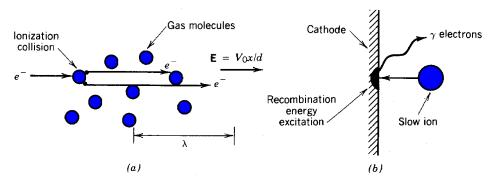
Figure 9.12 Processes in a gas-filled, high-voltage gap. (a) Electron migration in presence of a strong electric field showing electron acceleration, ionizing collision, and the mean free path. (b) Liberation of secondary electrons from a negative polarity electrode (cathode) by recombination of slow ions.
