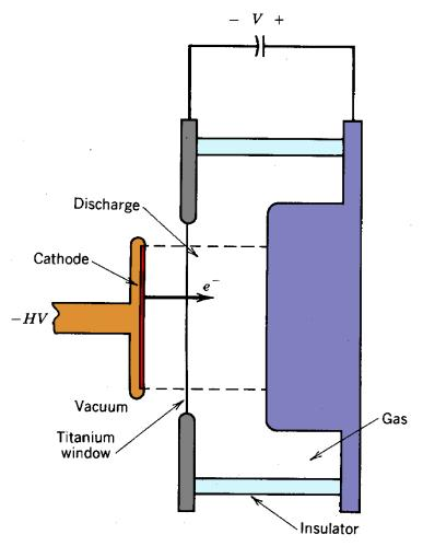
Figure 9.14 Electron-beam-controlled gas discharge laser.
