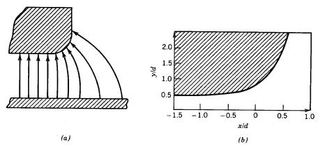
Figure 9.15 Electrode shaping. (a) Field enhancement at the edge of an electrode with a simple radius. (b) Electrode with a Rogowski profile.
