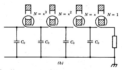
Figure 9.45 Saturable core magnetic switching. (a) Peaking capacitor circuit with magnetic output switch. (b) Multistage power compression circuit with uniform capacitors and ferromagnetic cores.
