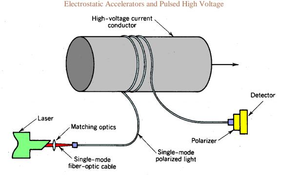
Figure 9.59 Current probe using Faraday rotation of laser-generated light in a fiber-optic cable.
