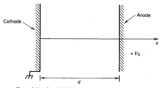
Figure 9.11 Gas-filled high-voltage gap, planar electrodes.
