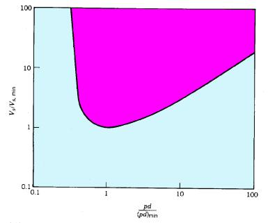
Figure 9.13 Normalized Paschen curve; sparking voltage versus the product of pressure and gap width.
