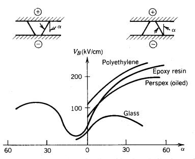
Figure 9.21 Insulator breakdown levels as function of insulator inclination angle for materials subject to fast voltage pulse (~ 30 ns). (Adapted from I. D. Smith, Proc. First Int. Symp. Discharges and Elec. Insul. in Vac., MIT, Cambridge MA, 1964, p. 261.)
