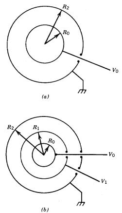
Figure 9.19 Geometry for calculating electric fields on spherical electrodes. (a) Two concentric spheres. (b) Concentric spheres with an equipotential shield.
