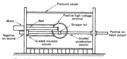
Figure 9.18 Schematic diagram of a tandem Van de Graaff accelerator.
