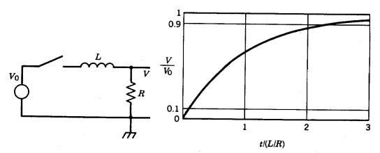
Figure 9.5 Time-dependent load voltage from a pulse generator with a series inductance.
