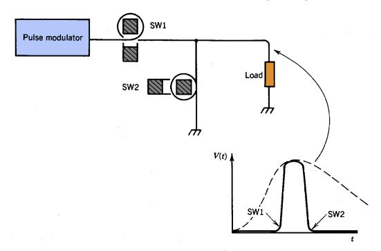
Figure 9.48 Pulse shaping with saturable core magnetic switches.
