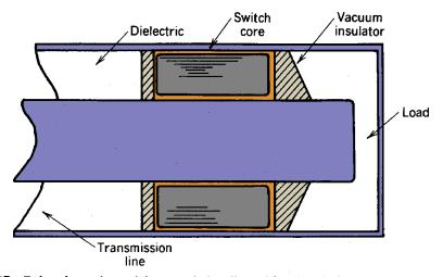
Figure 9.47 Pulse-charged coaxial transmission line with a low-inductance, saturable core magnetic output switch.
