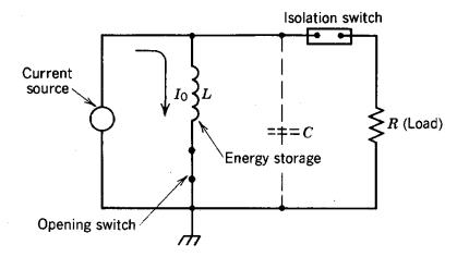
Figure 9.25 Pulse modulator with inductive energy storage and opening switch.
