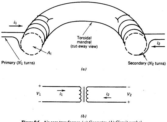
Figure 9.6 Air core transformer. (a) Geometry. (b) Circuit symbol.
