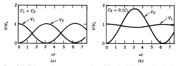
Figure 9.44 Voltage waveforms on storage capacitor and charged capacitor in a peaking capacitor circuit. (a)  $C_2 = C_1$ . (b)  $C_2 = 0.1C_1$ .
