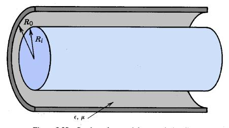
Figure 9.28 Section of a coaxial transmission line.
