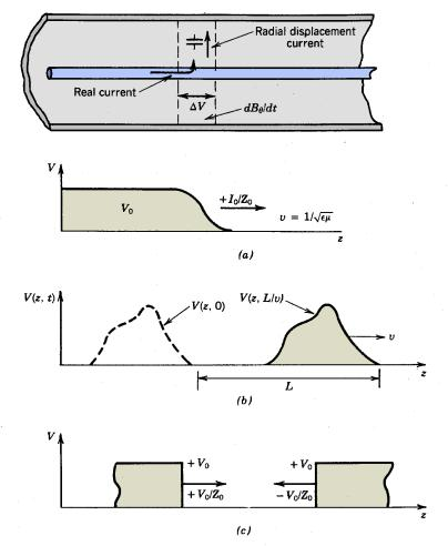
**Figure 9.30** Coaxial transmission line. (a) Distribution of voltage, real current, and displacement current for a sharp rising step pulse propagating along a transmission line. (b) Distributions of voltage on a transmission line at time t = 0 (dashed line) and time t = L/v (solid line). (c) Polarity conventions for positive voltage impulses traveling in the +z and -z directions.
