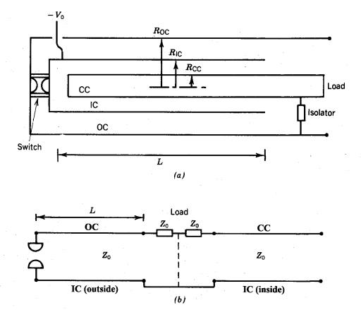
Figure 9.34 Nested coaxial transmission lines in the Blumlein configuration. (a) Schematic view and definition of quantities. (b) Equivalent circuit.
