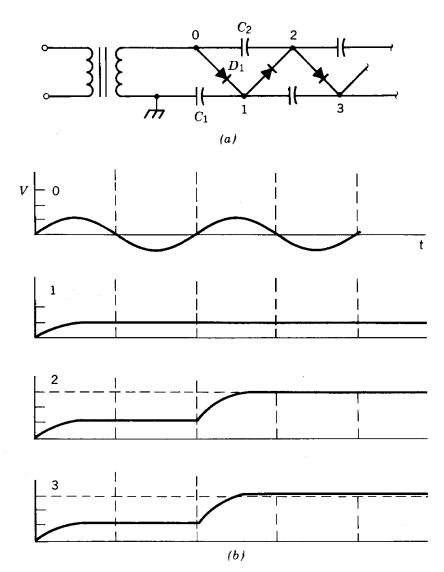
**Figure 9.10** (*a*) Voltage multiplication ladder network (Cockcroft–Walton accelerator). (*b*) Ideal voltage waveforms (neglecting the ac generator impedance) shown at various points of the network.
