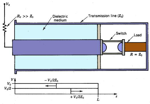
Figure 9.33 Coaxial transmission line used as a square-pulse generator.
