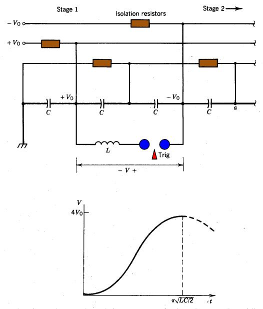
Figure 9.27 Circuit diagram of a typical LC generator, showing voltage at point a following switching through the external inductor.
