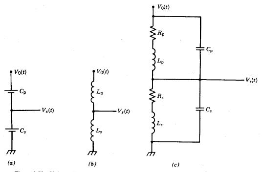
Figure 9.53 Voltage dividers. (a) Capacitive. (b) Inductive. (c) Balanced voltage divider.
