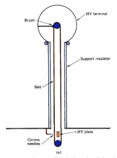
Figure 9.17 Van de Graaff accelerator. (a) Principle of operation. (b) Los Alamos National Laboratory, 7 MeV Van de Graaff accelerator, utilized as injector for 24.5 MeV tandem Van de Graaff accelerator facility. (Courtesy, J. R. Tesmer, Los Alamos National Laboratory.)
