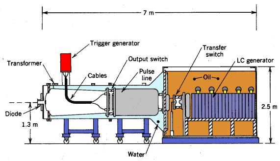
Figure 9.42 Neptune C, low-impedance pulsed power generator using overstressed water dielectric. (Courtesy H. Milde, Ion Physics Corporation.)
