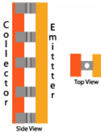
Figure 4.4-7: View of Holes in Ceramic Spacers for Cesium Passage
