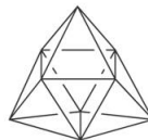
n = 9 Tricapped trigonal prism
