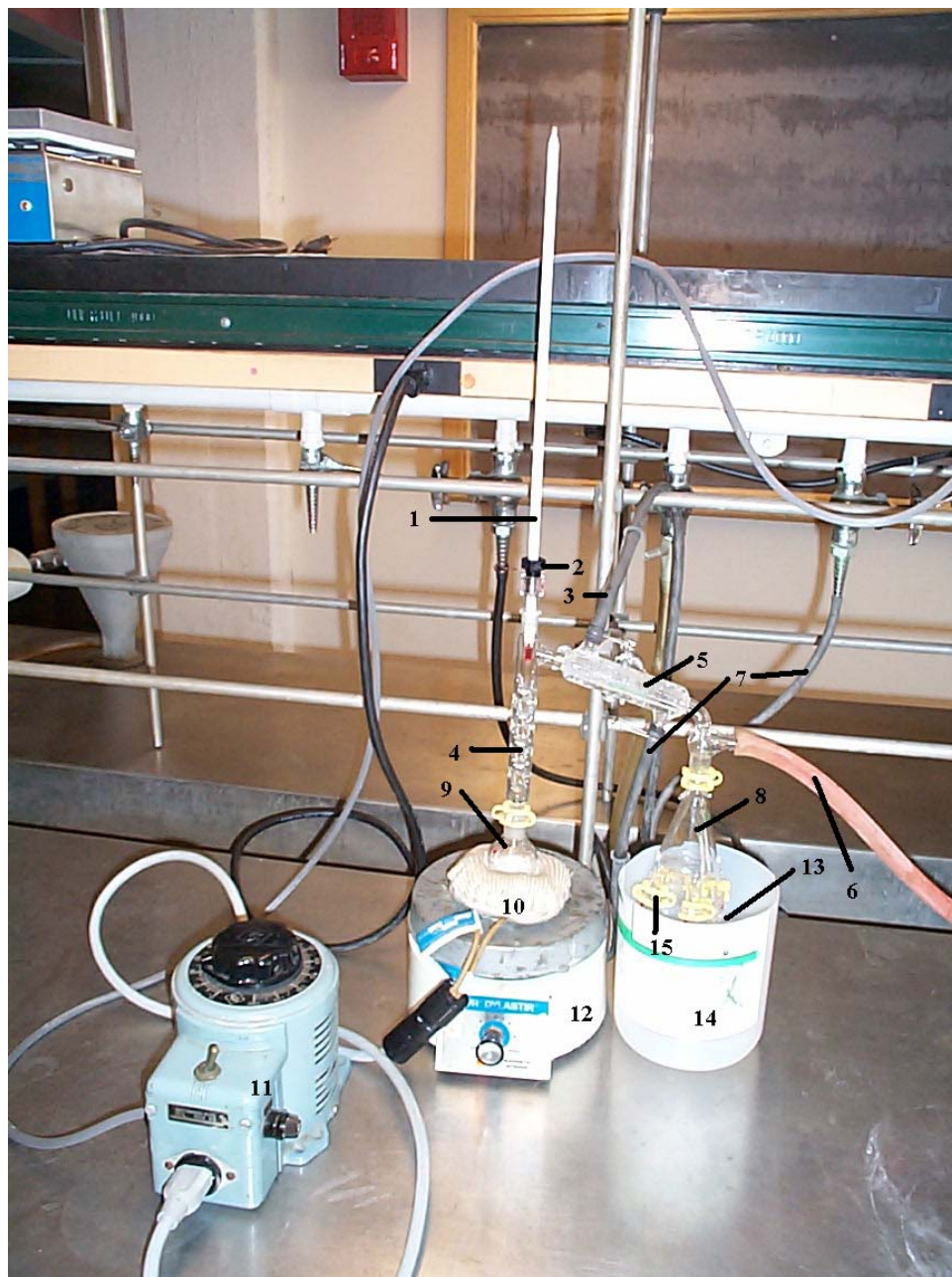
Figure 2. Apparatus used for Vacuum Distillation
