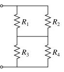
The Thévenin resistance of this new circuit is just the series combination of  $R_1||R_2$  and  $R_3||R_4$  which is equal to
