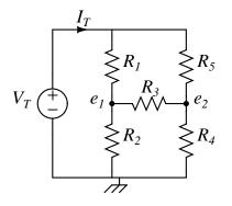
We know that the current  $I_T$  is equal to the sum of the currents down through the resistors  $R_2$  and  $R_4$ . This can be written as  $I_T = G_2 e_1 + G_4 e_2$ , where  $G_2$  and  $G_4$  are the conductances
