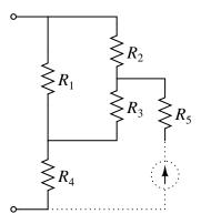
The resistor  $R_5$  does not impact the Thévenin resistance, because one of its terminals is not connected to the rest of the network now that the current source has been removed.  $R_2$  and  $R_3$  are in series, in parallel with  $R_1$ . All of this is in series with  $R_4$ . The resulting resistance is
