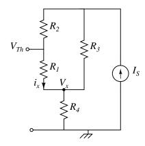
It is clear that the current running through  $R_4$  is equal to  $I_S$ . We know, then, that  $V_x = I_S R_4$ . We also know that  $V_{Th} = V_x + i_x R_1$ . The current  $i_x$  can be found using the current divider relationship:
