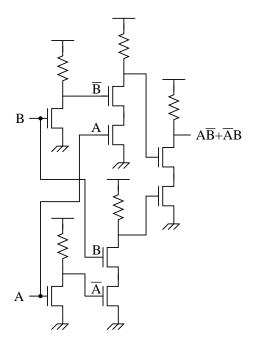
(ii) The circuit implemented with NOR and NOT gates is
