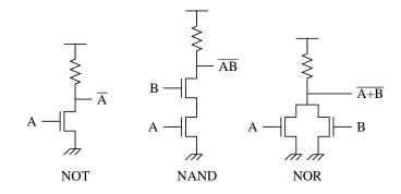
We can use these building blocks and connect them according to the diagrams in Part (A) to find the following implementations.
