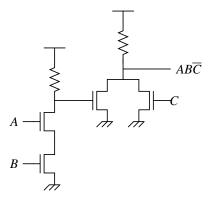
(C) This expression is a little more challenging to synthesize with no more than four MOSFETs and two resistors. Notice that the output should be high when either AB or C is high. We can synthesize a circuit which has the opposite behavior, that is the output is low when AB or C is high. That circuit is
