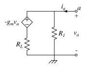
The Thévenin resistance is  $R_{Th} = \frac{v_a}{i_a}$ . Write KCL at the node *a* to obtain
