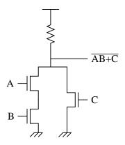
Add an inverter to it's output, and we get the desired logic function. This circuit is
