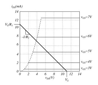
(b) For this circuit,  $v_{DS} = V_S - v_O = V_S - R_2 i_{DS}$ . When  $i_{DS} = 0$ ,  $v_{DS} = V_S$ . When  $v_{DS} = 0$ ,  $i_{DS} = \frac{V_S}{R_2}$ . The slope of this line is  $-\frac{1}{R_2}$ . It is plotted on the figure below.
