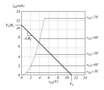
(c) For this circuit,  $v_{DS} = V_S - (R_1 + R_2)i_{DS}$ . When  $i_{DS} = 0$ ,  $v_{DS} = V_S$ . When  $v_{DS} = 0$ ,  $i_{DS} = \frac{V_S}{R_1 + R_2}$ . Thes slope of this line is  $-\frac{1}{R_1 + R_2}$ . It is plotted on the figure below.
