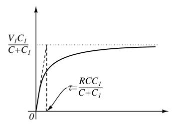
If the same energy is to end up in  $C, v(\infty)$  must be equal for both circuits. This means
