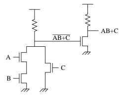
Again, in the inverter we just replace the pullup resistor with a PFET. In the first gate's NFETs, A and B are in series, in parallel with C. The PFETs will be A and B in parallel, in series with C, as shown below.
