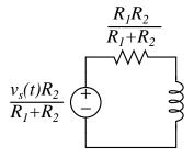
(a) This input is just a unit step. The current through an inductor must be continuous unless an infinite voltage is applied across it, so we know the voltage step must appear across the inductor, not the resistor. Given this:
