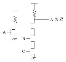
In the inverter just replace the pullup resistor with a PFET. The NFETs in the second stage are all in series. The corresponding PFETs get placed in parallel in place of the pullup resistor, as shown below.
