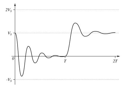
(B) We know that once the output of the circuit becomes a valid high output for a valid low input, it should not leave the valid high output region. This means that the lowest ringing trough when the output switches high must be  $> 0.8V_S$ .
