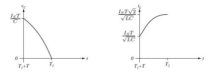
(E) Here is a sketch of  $v_C(t)$  and  $i_L(t)$  for  $0 < t < T_2$ .
