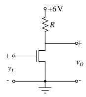
Assume that the FET has an "on" resistance of  $200\Omega$  and a threshold voltage of  $2.5 \pm 0.1$ V. The  $\pm 0.1$  deviation accounts for device-to-device variations. The static discipline for the chip in which this FET will be used is
