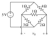
**Problem 1.6:** For the circuit below, write a set of three KCL equations sufficient to solve for the node to reference voltages  $e_1, e_2$ , and  $e_3$ . Express your equations in the form:
