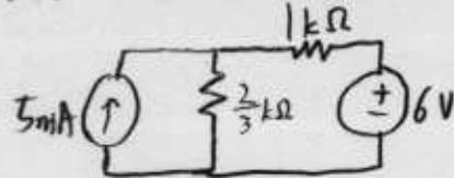
We can switch to Thevenin equivalent one more time and add the two resistors in series.
