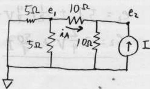
F.) First combine the two  $5\Omega$  resistors to form a  $2.5\Omega$  resistor. This results in the circuit below. Since it flows through the  $2.5\Omega$  and  $10\Omega$  resistor in series we can use a current divider to get  $i_A$ .
