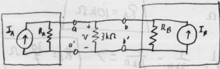
When the  $3\text{k}\Omega$  resistor is replaced by a short circuit,  $i_A = -I_A$  and  $i_B = -I_B$ ; therefore,  $I_A = 6\text{mA}$  and  $I_B = -2\text{mA}$ . Combining the two current sources and the two unknown resistors results in the following circuit.
