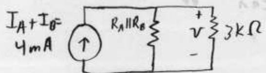
We know that with the  $3\text{k}\Omega$  resistor in the circuit  $V = 6\text{V}$ . From this we can determine the parallel combination of  $R_A$  and  $R_B$ .
