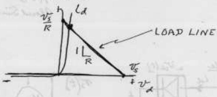
Explain the common joint is where the circuit operates. Also, explain what happens when  $v_s$  is changed, and when the value of  $R$  is changed, holding  $v_s$  constant
