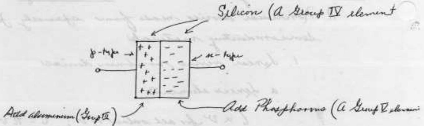
A semiconductor material (e.g., silicon or germanium) is injected with a small amount of another element (about 1 part per million, by weight).
