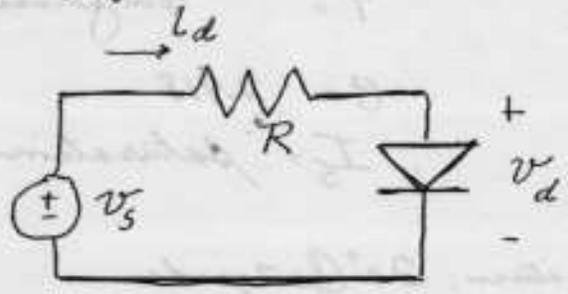
The key is to find a representation of the diode that makes the circuit easy to analyze. The representation is called a model.
