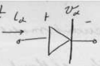
We said the  $I_d, V_d$  characteristic of the diode is nonlinear.
