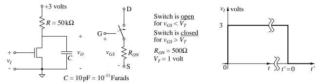
For t < 0 the input voltage  $v_I$  is zero. At t = 0  $v_I$  changes instantly to  $v_I = 3V$ . A long time later at a time t' = 0, the input voltage changes instantly to zero, as shown in the sketch above.
