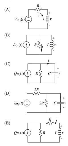
**Problem 7.2:** Pick any three of the five circuits shown in Problem 7.1. For each of your choices, sketch and dimension the indicated voltages and currents for t > 0. Evaluate time constants in terms of circuit elements. Label your drawings clearly, including the designation (A), (B)  $\cdots$  (E) of your choices.
