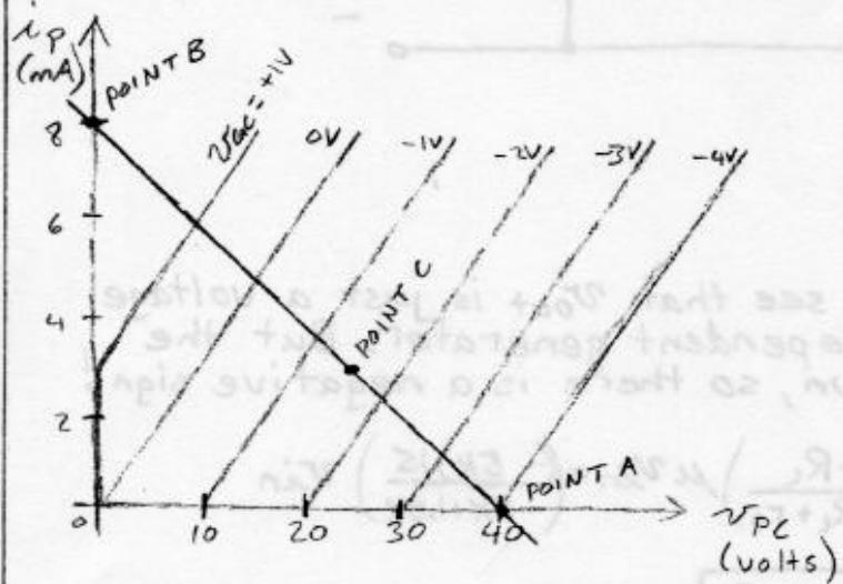
The circuit constrains the solution to lie on the loadline. We want  $i_p = 3mA$ , which is Point C.
