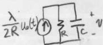
at  $t=0^+$  an impulse of charge is dumped on the capacitor.
