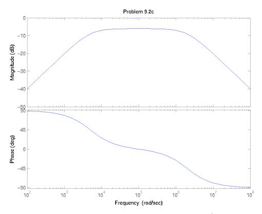
D) From the above graph, the magnitude is almost flat for roughly  $10^4$  rad/s <  $\omega$  <  $10^6$  rad/s or 1.6 kHz < f < 160 kHz
