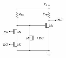
**Answer:** Because  $R_{\rm ON} \ll R_{\rm PU}$ , we can approximate  $R_{\rm PU} + nR_{\rm ON} \approx R_{\rm PU}$ , where n is small ( $\leq 2$  for this problem). Also, we can say that the capacitor  $C_{\rm GS}$  will fully charge or discharge in each switching period T, because  $T \gg R_{\rm PU}C_{\rm GS}$ .
