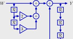
We can "reuse" 2 delays by commuting the left and right parts of this network. Next compute w[n] which is the first difference of x[n]:
