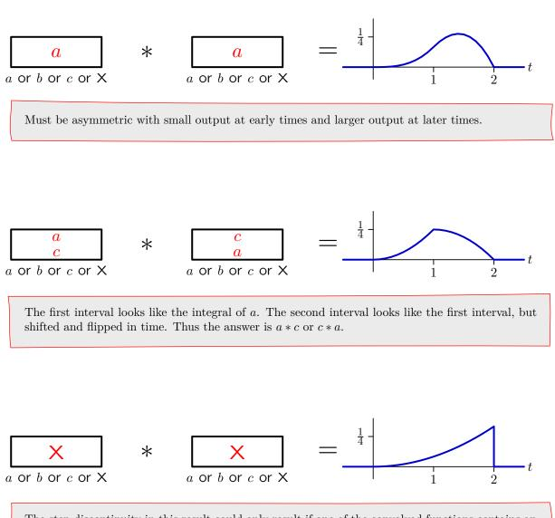
The step discontinuity in this result could only result if one of the convolved functions contains an impulse.
