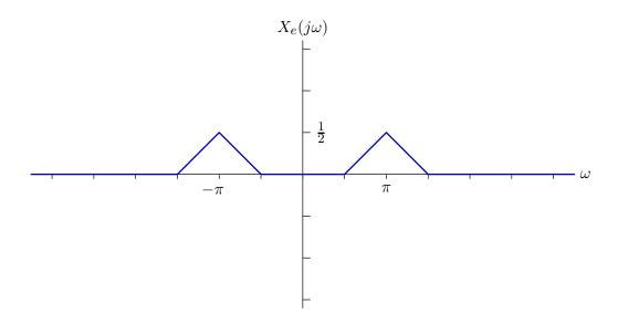
**Part c.** Is it possible to adjust T so that  $X_e(j\omega)$  has the following form when  $\omega_m = 5\pi$ ?
