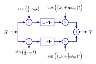
Assume that each lowpass filter (LPF) is ideal, with cutoff frequency  $\omega_m/2$ . Also assume that the input signal has the following Fourier transform.
