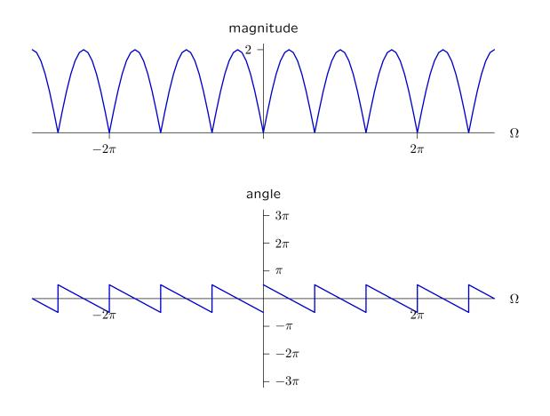
$$H(e^{j\Omega}) = 1 - e^{-j3\Omega} = e^{-j3\Omega/2} \left( e^{j3\Omega/2} - e^{-j3\Omega/2} \right) = j2e^{-j3\Omega/2} \sin\frac{3\Omega}{2}$$
