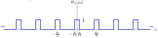
Since y[n] = x(3n),  $w_1(t)$  is equal to x(t) times and infinite train of unit impulses separated by T = 3 seconds:
