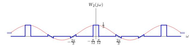
The signal  $w_2(t)$  can be derived by convolving  $w_1(t)$  with a signal  $s(t) = \frac{1}{3}\delta(t-1) + \frac{1}{3}\delta(t) + \frac{1}{3}\delta(t+1)$ .
