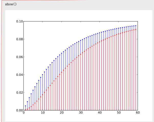
Since the rate of influx to tank 2 starts more slowly than that to tank 1, the height in the second tank gets started more slowly than that in the first. Ultimately, the heights of water in both tanks approach the same value.
