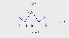
From the plot, it is clear that  $x_e(t) = 0$  if |t| > 2 or |t| = 1. Since x(t) is defined to be zero at  $t = \pm 2$ , we should include those points as well, so  $|t| \ge 2$  or |t| = 1.
