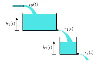
The rate of flow out of each tank is proportional to the height of the water in that tank:  $r_1(t) = k_1 h_1(t)$  and  $r_2(t) = k_2 h_2(t)$ , where  $k_1$  and  $k_2$  are each  $0.2 \text{ m}^2$ /second. Both tanks have heights of 1 m. The cross-sectional area of tank 1 is  $A_1 = 4 \text{ m}^2$  and that of the second tank is  $A_2 = 2 \text{ m}^2$ . At time t = 0, both tanks are empty.
