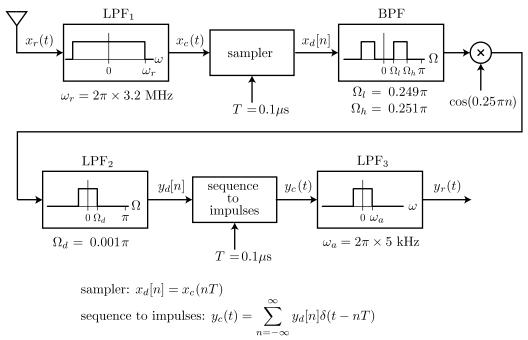
**Part a.** Determine the center frequency  $f_c$  for the AM station that this receiver will detect.
