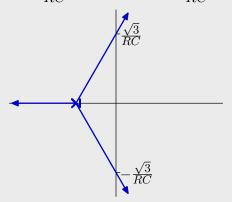
The point of marginal stability is where the root locus crosses the  $j\omega$  axis. This occurs when the real part of  $-1 + \sqrt[3]{K}e^{j\pi/3}$  equals zero:
