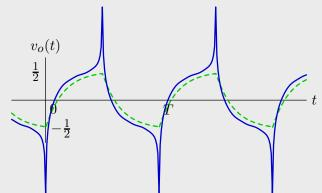
The asymmetry in the "charging" and "discharging" portions of the RC response is even more pronounced than before. Because the magnitudes of the higher harmonics are not attenuated, they now accumulate to make a substantial peak that was not seen in the RC response. We can understand the large overshoot as follows. Each harmonic component in the square wave is a sinusoid:
