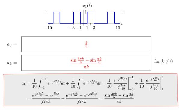
**b.** Determine the Fourier transform of the following signal, which is zero outside the indicated range.
