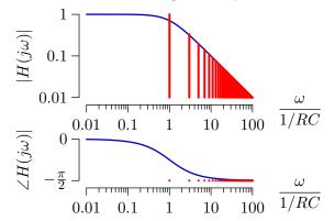
The RC filter has two effects: (1) The amplitudes of the Fourier components of the input (vertical red lines in upper panel) are multiplied by the magnitude of the frequency response  $(|H(j\omega)|)$ . (2) The phase of the Fourier components (red dots in lower panel) are shifted by the phase of the frequency response  $(\angle H(j\omega))$ .
