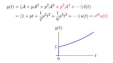
Making p negative makes the output converge (instead of diverge).
