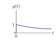
Making p negative makes the output converge (instead of diverge).
