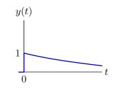
Making p negative makes the output converge (instead of diverge).
