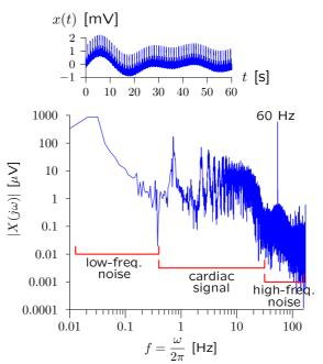
Filter design: low-pass filter + high-pass filter + notch.
