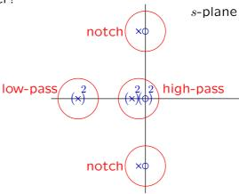
Filtering is a simple way to reduce unwanted noise.
