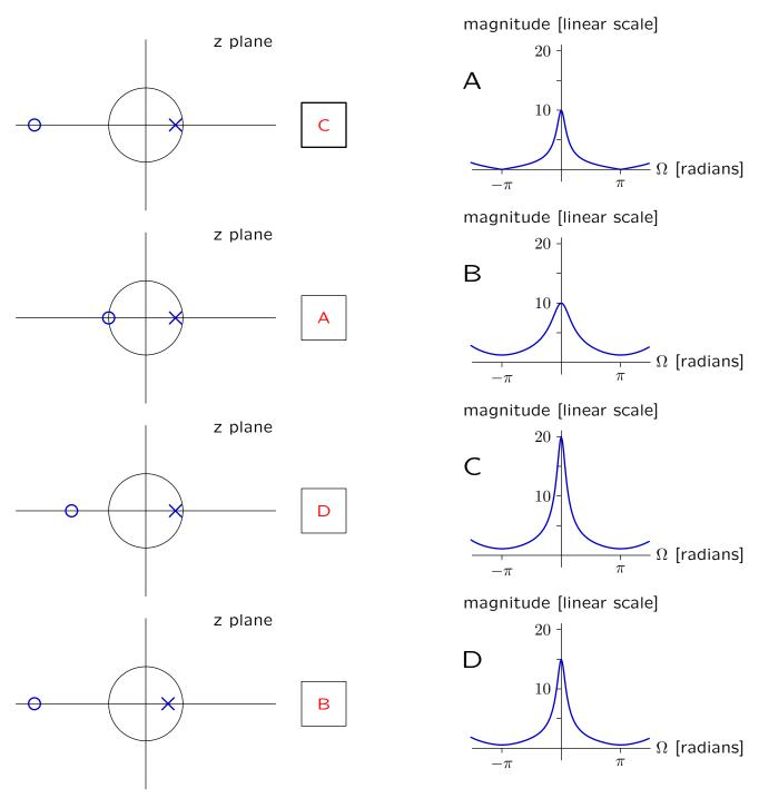
**Part b.** Each pole-zero diagram below shows the unit circle (radius 1) as well as the pole ( $\times$ ) and zero (o) of a **discrete-time**, linear, time-invariant system of the form
