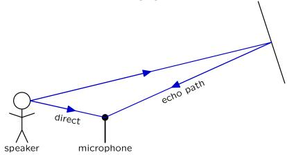
We can represent this recording situation as a linear, time-invariant system, with the speaker's voice as the input and the recorded microphone signal as the output. Assume that the impulse response of this system is
