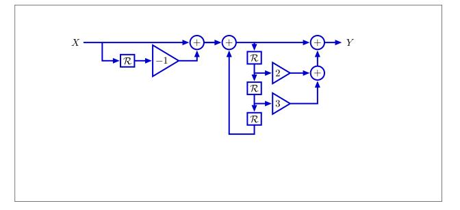
First find a system whose unit-sample response is the desired sequence. The periodicity of 3 suggests that y[n] depends on y[n-3]. To get the correct numbers, just delay the input and weight the delays appropriately. The resulting difference equation is
