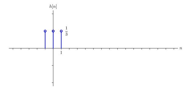
$$\frac{Y}{X} = K \frac{\left(z + \frac{1}{2} - j\frac{\sqrt{3}}{2}\right)\left(z + \frac{1}{2} + j\frac{\sqrt{3}}{2}\right)}{z} = K \frac{\left(z + \frac{1}{2}\right)^2 + \frac{3}{4}}{z} = K \frac{z^2 + z + 1}{z} = K \left(z + 1 + z^{-1}\right)$$
