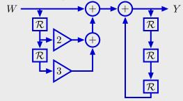
We can "reuse" 2 delays by commuting the left and right parts of this network.
