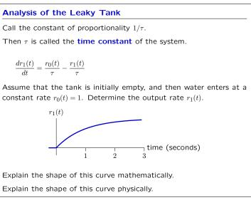
Leaky Tanks and Capacitors Although derived for a leaky tank, this sort of model can be used to represent a variety of physical systems. Water accumulates in a leaky tank.  $r_0(t)$
