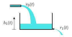
Assume linear leaking:  $r_1(t) \propto h_1(t)$
