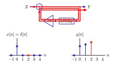
The effect of feedback can be visualized by tracing each cycle through the cyclic signal paths.
