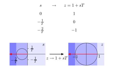
DT stability: CT pole must be inside circle of radius  $\frac{1}{T}$  at  $s = -\frac{1}{T}$ .
