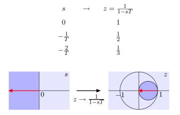
The entire left half-plane maps inside a circle with radius  $\frac{1}{2}$  at  $z = \frac{1}{2}$ . If CT system is stable, then DT system is also stable.
