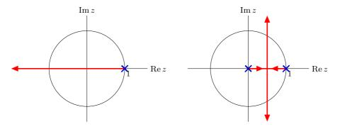
Fastest response without delay: single pole at z = 0.
