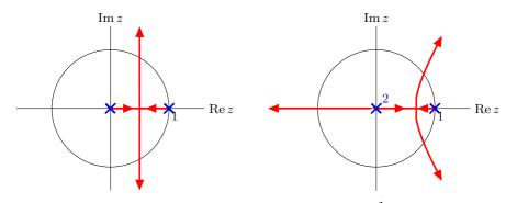
Fastest response with delay: double pole at  $z = \frac{1}{2}$ .
