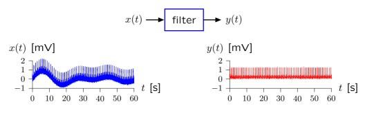
We can identify the "noise" by breaking the electrocardiogram into frequency components using the Fourier transform.
