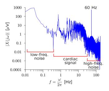
Filter design: low-pass filter + high-pass filter + notch.
