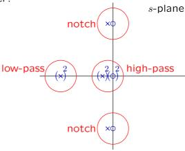
By placing the poles of the notch filter very close to the zeros, the width of the notch can be made quite small.
