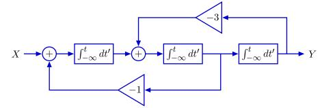
**Part a.** Is it possible to represent this system with a linear differential equation with constant coefficients?
