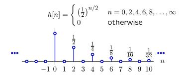
**Part a.** Is it possible to represent this system with a finite number of poles?
