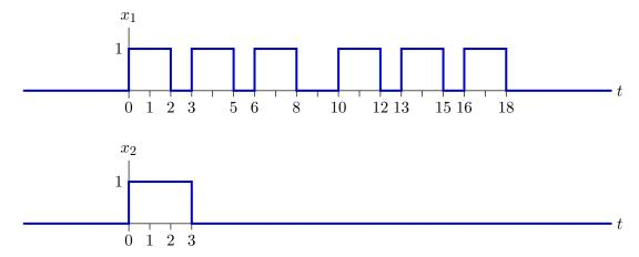
Plot the result of convolving  $x_1(t)$  with  $x_2(t)$ . Make sure that the important break-points are clear.
