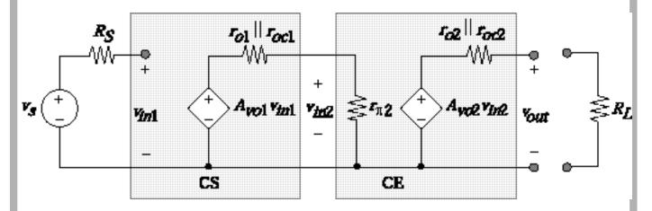
However, inter-stage loading degrades gain:
