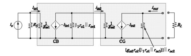
$$\mathbf{R}_{\text{out}} = \mathbf{R}_{\text{out}2} = \mathbf{r}_{\text{oc}2} \parallel \left[ \mathbf{r}_{\text{o}2} \left( 1 + \mathbf{g}_{\text{m}2} \mathbf{R}_{\text{out}1} \right) \right]$$
