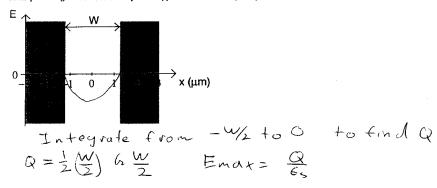
1b) (5 points) Sketch the electrostatic potential in the depletion region. Provide an expression for the value of the electrostatic potential at x=0. Use the depletion approximation and express your answer in terms of W and G.
