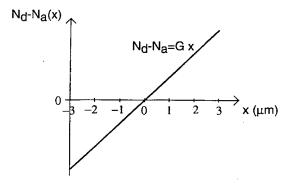
This doping distribution results in a space charge layer (a depletion layer) of width W that separates two quasi-neut regions. The resulting charge density distribution is sketched below.
