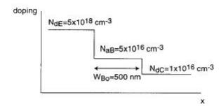
The width of the metallurgical base (the entire extent of the p base) is  $W_{Bo} = 500 \ nm$ . The emitter cross-sectional area is  $A_E = 10 \ \mu m^2$ . This transistor is biased such that the collector current  $I_C = 10 \ mA$  and the base-collector voltage  $V_{CB} = 5 \ V$ . The electron diffusion coefficient in the base is  $D_n = 10 \ cm^2/s$ . Assume that the depletion width of the emitter-base junction is negligible.
