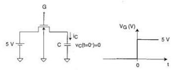
At  $t=0^-$ ,  $V_G=0$  V, and the voltage across the capacitor  $v_G(t=0^-)=0$ . At t=0, the gate voltage rises abruptly to  $V_G=5$  V and remains there. The transistor parameters are as follows:  $L_g=1$   $\mu m$ ,  $W_g=2$   $\mu m$ ,  $\mu_n C_{\sigma\pi}=50$   $\mu A/V^2$ ,  $V_{To}=1$  V,  $\gamma=0.6$   $V^{1/2}$ ,  $\phi_p=-0.4$  V.
