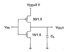
la) (5 points) Calculate  $V_{Tn}$  so that  $V_M = 1.5 V$ .
