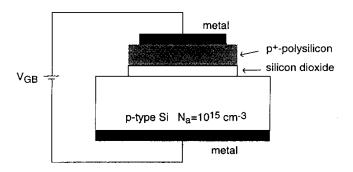
The capacitance-voltage curve for this device is shown below:
