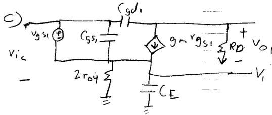
$$V_{o1} = \frac{-g_m R_D}{1 + 2g_m r_{o4}} v_{i,c}$$
