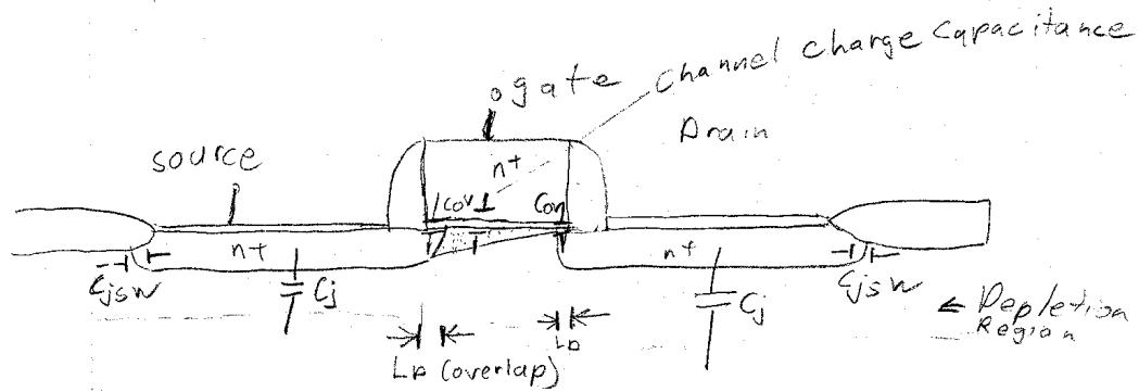
$$C_{GS} = \text{channel charge} + \text{overlap capacitance}$$
