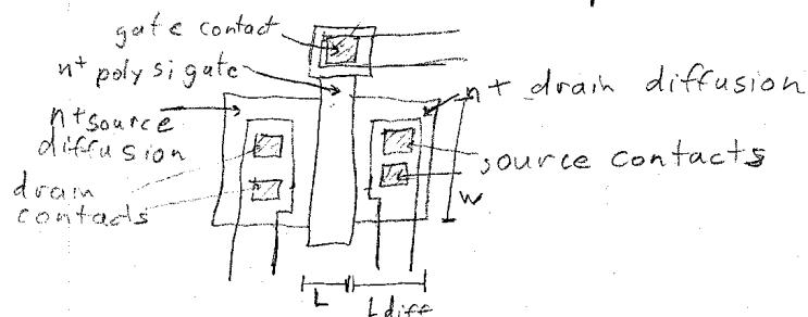
$$C_J = W L_{diff} \sqrt{\frac{q \epsilon_s N_a}{2(\phi_0 - V_{BS})}} \quad \text{rev, braided pn-jct} \quad V_{BS} < 0$$
