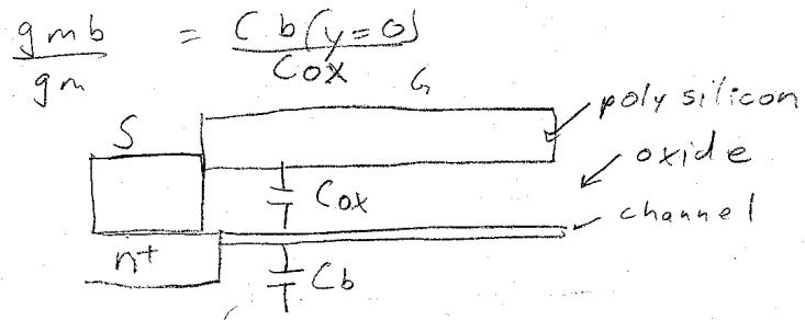
$$C_{ox} = \frac{Q_{channel}}{V_{GC}} \quad C_b = \frac{Q_{channel}}{V_{BE}}$$
