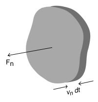
Relationship between particle flux and velocity:
