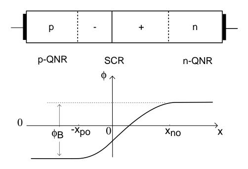
Question 1: If I apply a voltmeter across diode, do I measure  $\phi_B$ ?
